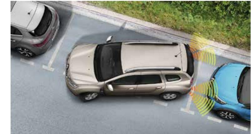
**Rear Park Distance Control.** To make parking manoeuvres easier. The parking distance control system warns you of obstacles situated behind the vehicle by a sequence of beeps which speed up the closer you are to them.
