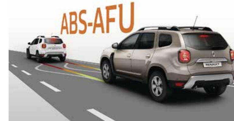
**(ABS) Anti-lock Braking System** with **(EBD) Electronic Brake Force Distribution**, in conjunction with **(EBA) Emergency Brake Assist**: makes it possible to maintain control over the trajectory in the event of heavy braking.
