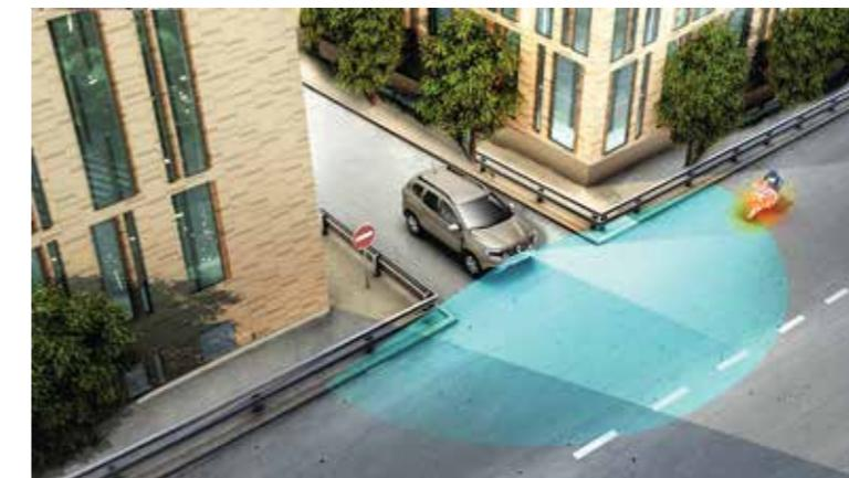
**MultiView Camera.\*** Connected to the MediaNav system, the MultiView Camera shows the images from Duster's four on-board cameras. It is triggered by reverse gear or by a simple touch of the dedicated button.
