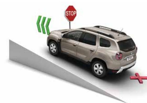
**(HSA) Hill Start Assist.** Starting the car on steep slopes is no longer a worry. When you take your foot off the brake, hill-starting assist takes over and holds the vehicle steady for two seconds. This gives you time to accelerate normally without stalling or rolling back.
